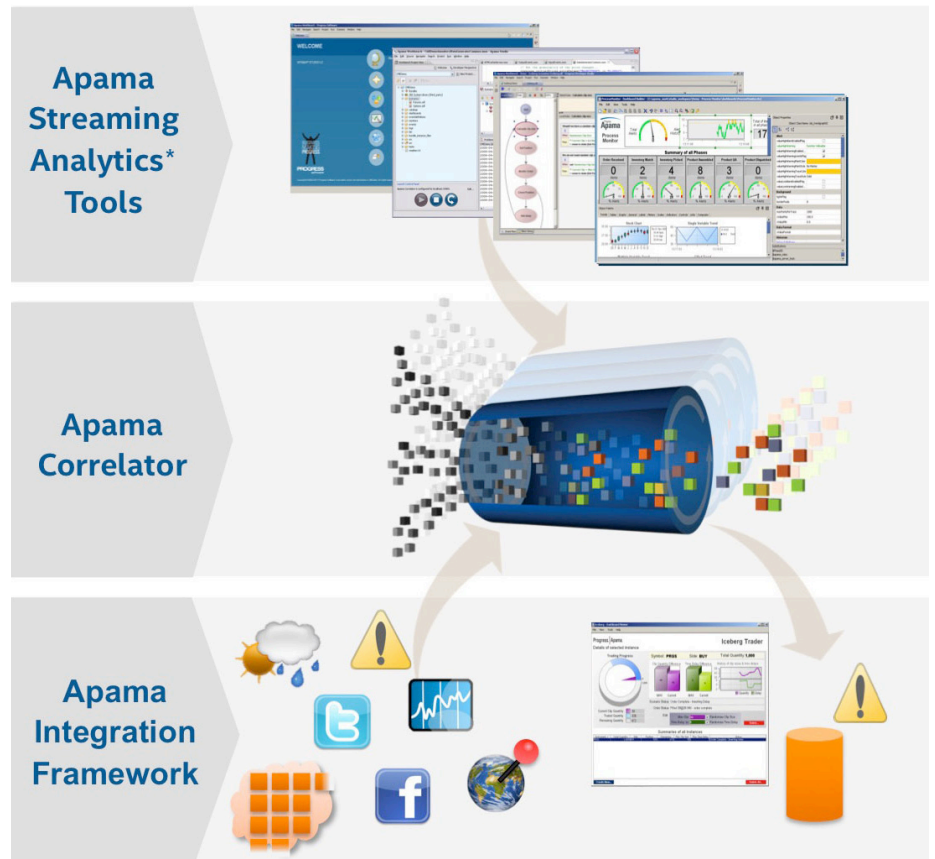
Figure 1. Components that comprise the Apama Streaming Analytics* event-processing architecture
